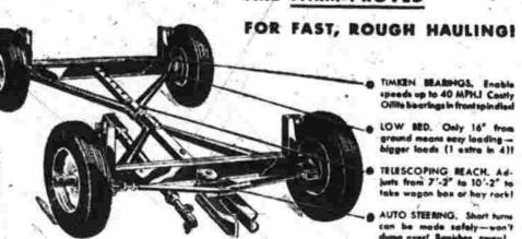
TIMICEN BEARINGS, Engble speeds up to 40 MPH.I Cost ground means easy leading -bigger loads (1 extra in 4)! justs from 7'-2" to 10'-2" t take wagon bax or hay rock AUTO STEERING. Short turns
